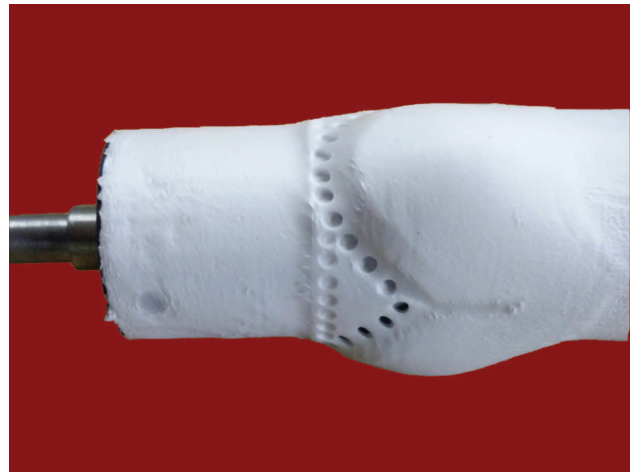
Figure 8: The laser welded heart valve scaffold, view from side.
