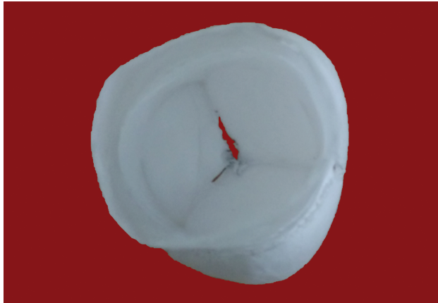
Figure 7: The laser welded heart valve scaffold, view from above.
