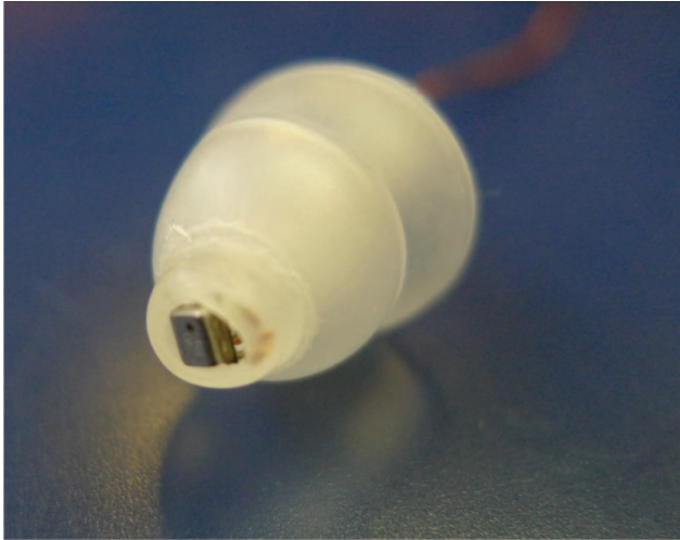
Figure 1: Air pressure sensor integrated in a silicone in-ear plug.
