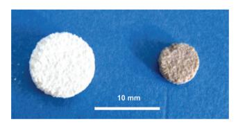
Figure 2: Green part and sintered part of M1.
