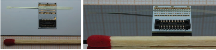
Figure 2: Flip-chip bonded 3D- \mu ECoG-MEA to PCB with SAC305.
