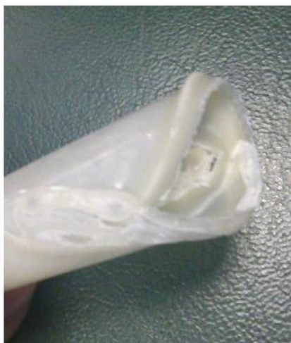
Photo of the poly(DL-Lactide-co ethylene brassylate) polymer, which was catalyzed with iron(III)perchlorate
