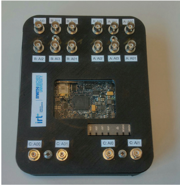
Figure 5: Hardware interface unit to be used with ModeliChart.
