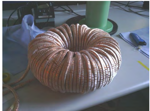
Image 7 Toroidal coil with 104 windings of a 7.5 \text{ mm} thick litz wire resulting in an inductance of 164 \text{ }\mu\text{H} and 43 \text{ m}\Omega at 25 \text{ kHz} .
