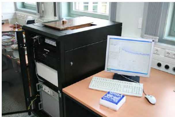
Image 1 Magnetic particle spectrometer MPS (Fork Labs project @ University of Lübeck ).
