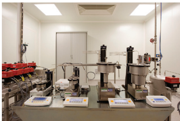
Figure 9: The weighing section of the CETIAT facility inside the clean room.
