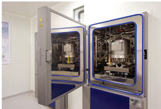
Figure 7: CETIAT facility. The water tank in the thermostatic chamber.
