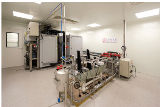
Figure 6: CETIAT clean room with the measuring line.
