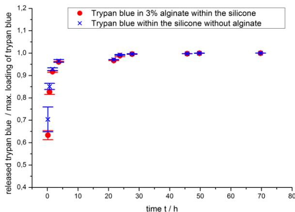
Figure 2: Diffusion of trypan blue out of the composite
