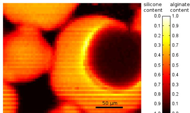
Figure 1: Confocal Raman Microscopy image of an alginate-silicone-composite with interpenetrating network
