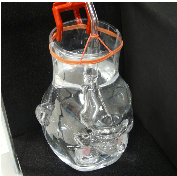
Figure 2: Assembled head phantom including eye balls and the air-filled glass insert (nasal cavities and sinuses).
