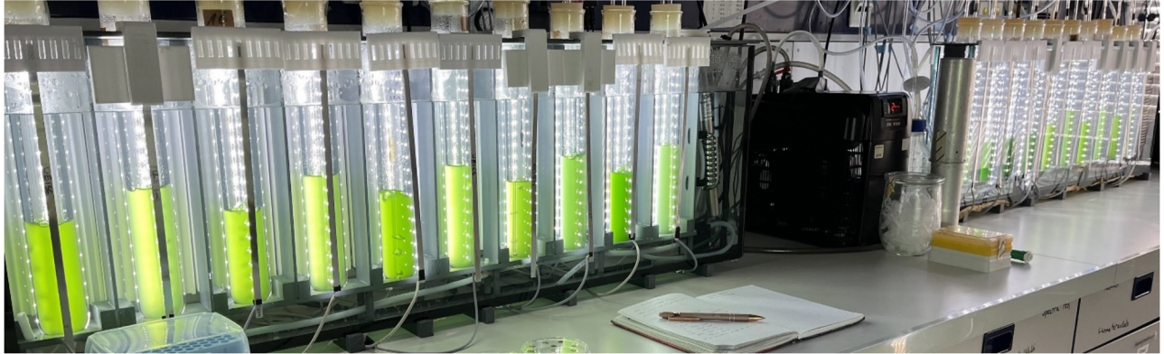
Figure 2: Photobioreactor for research. Flexible regulation and control of growth parameters for an optimal study of microalgae.
