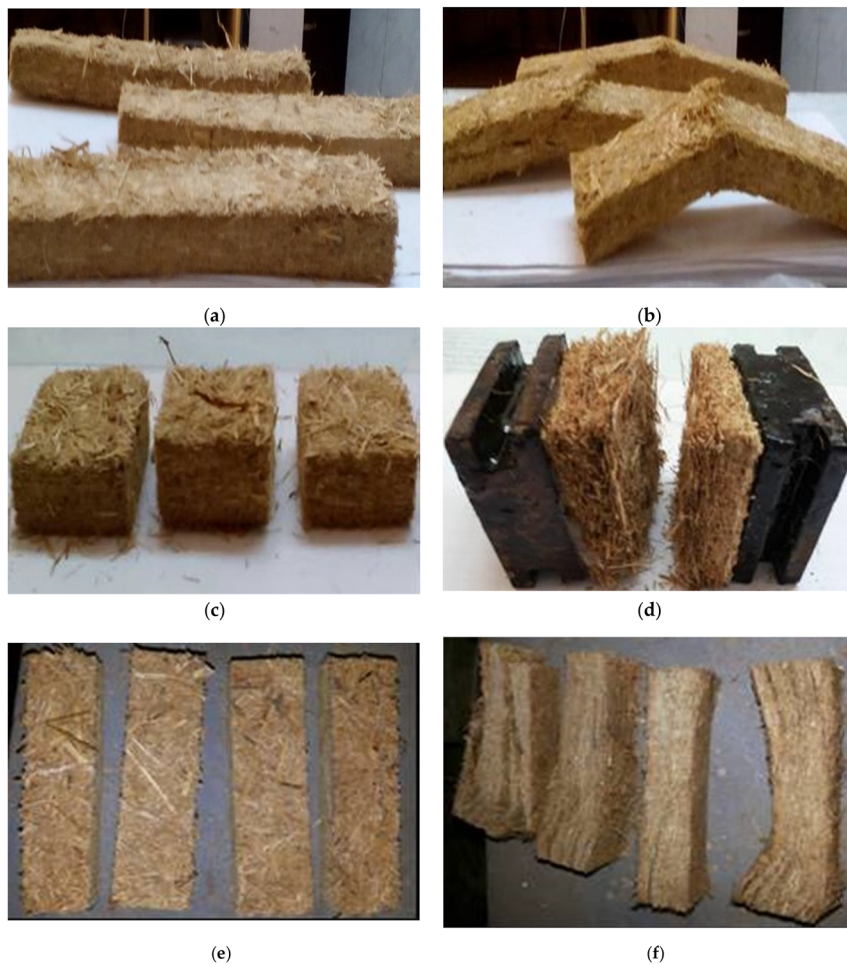
Figure 2: Test specimens of particleboard before (a, c, e) and after (b, d, f) the test procedure [3]: (a, b) static bending test; (c, d) tensile test; (e, f) compressive strength test.
