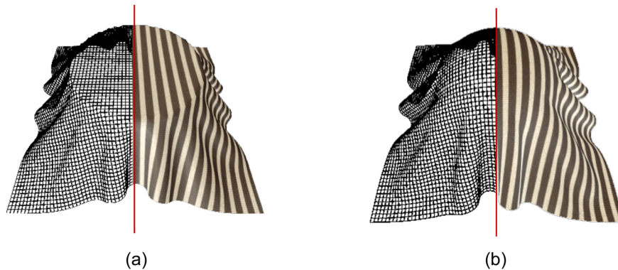
Figure 3. Virtual fabric. (a) Fabric with a disc supporter. (b) Fabric with a sphere supporter. Note: A disc supporter is achieved through the process of vertical projection, specifically by projecting the particles that surpass the disc above it. While a sphere supporter is obtained by the radius projection, that is, to project the particles inside the sphere along the radius onto its surface.
