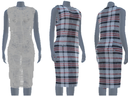
Figure 12. Effect of contact simulation with body slices (mesh and rendered). Note: The implementation is conducted on the Windows operating system taking advantage of OpenGL.
