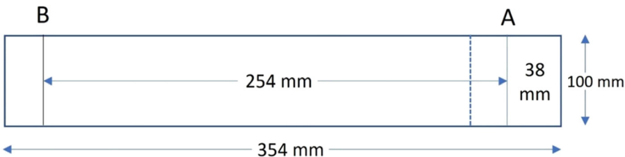
Figure 2. Sample specification of horizontal flammability test.
