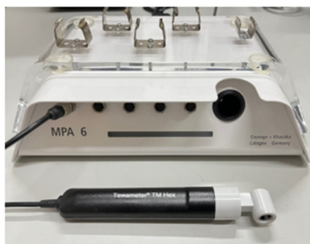
Figure 5. MPA6 multi-probe test system and the Tewameter TM Hex skin moisture loss test probe.
