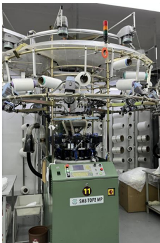
Figure 1. Saint-Tony SM8-TOP2 MP seamless circular knitting machine.
