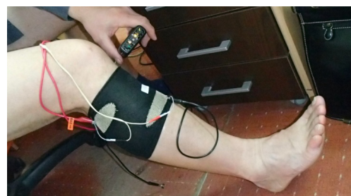
Figure 12. Tests performed with the knitted electrodes
