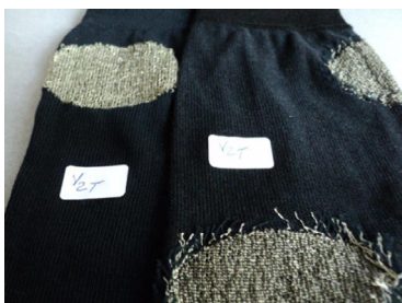
Figure 11. Functional textile with knitted electrodes
