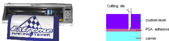
Figure 2. Roland GX-24 Vinyl Cutter [4] and a way of cutting to the depth of the carrier layer.
