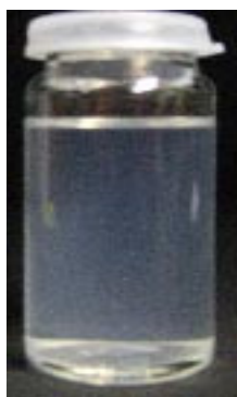
Figure 1. Image of a ZnO sol taken ten weeks after synthesis. The absence of any precipitations proves the excellent stability of the colloidal solution.
