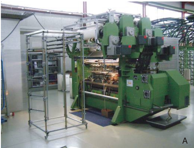
Figure 3. Double-needlebar raschel machine (A); developed yarn supplying system (B).
