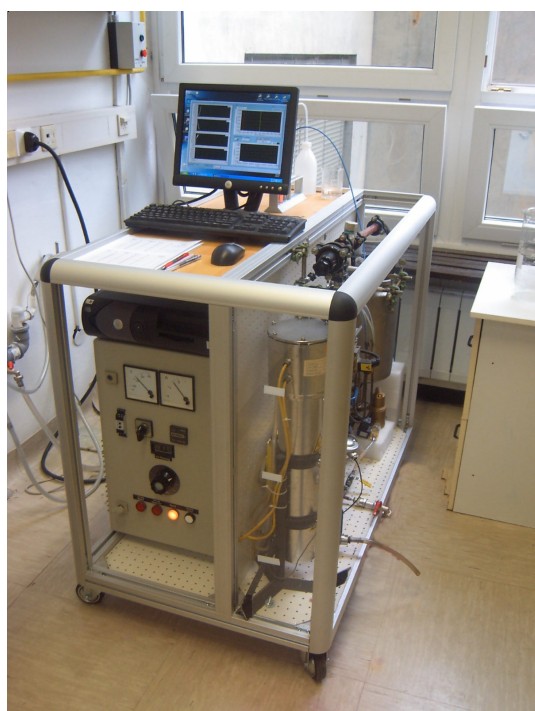
Figure 4. Photo of the UV/H 2 O 2 laboratory scale reactor for textile waste water decolouration.
