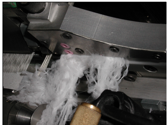
Figure 8. 'Air covered' yarn clogging the stretch nozzle.
