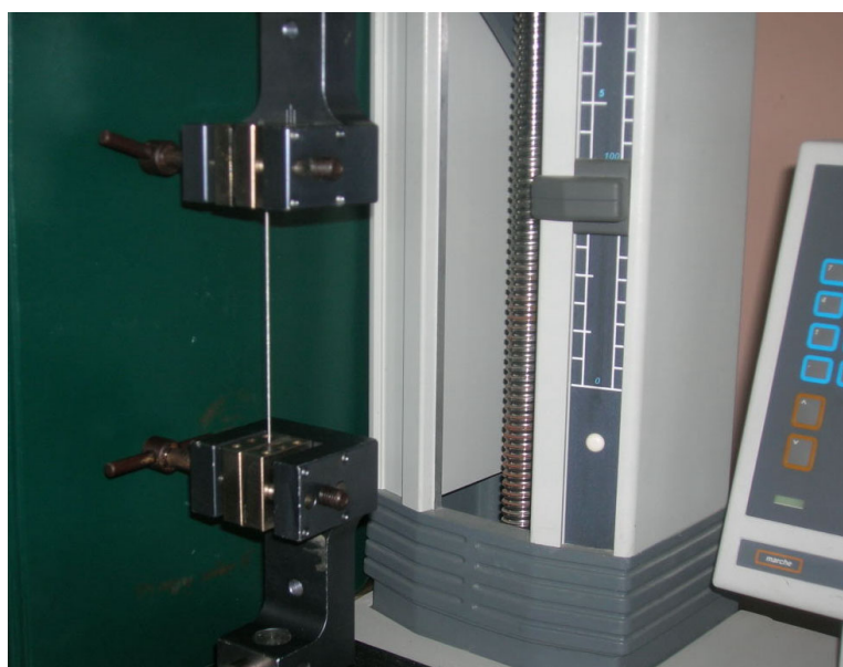
Figure 2. Dynamometer for breaking strength measurements
