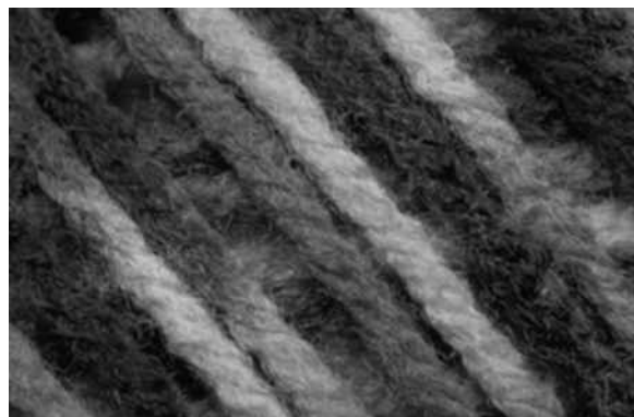
Figure 4. Image of the woven fabric from Figure 2 after the operation of levelling the histogram and using the procedure of the averaging mask (elaborated by the authors)
