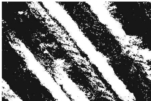
Figure 6. Image of the woven fabric from Figure 2 after the threshold procedure (elaborated by the authors)
