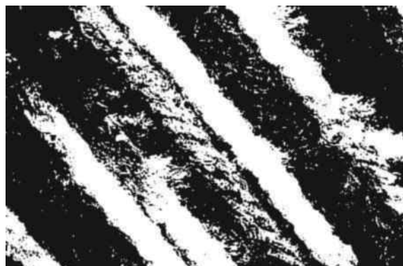
Figure 9. Image of the woven fabric from Figure 2 after application of the erosion and dilatation procedure on the mask previously processed by the threshold procedure (elaborated by the authors)
