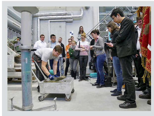
Figure 4: Workshop for rheological measurements with Sliper and eBT-V at the concrete laboratory of the OTH Regensburg.
