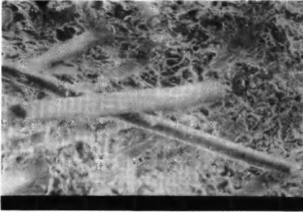
Fig. 6: General view of both parallel and perpendicular glass fibres in the composite (9G12)
