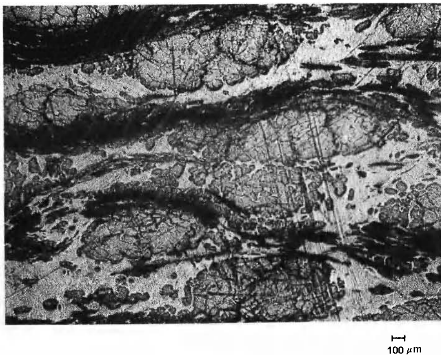
Fig.1: Weave structure of the jute fibre reinforced composite
