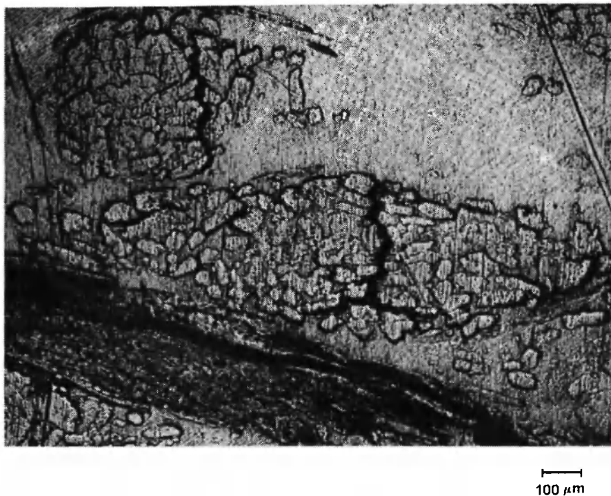
Fig.9: Micrograph of the jute/polyester laminate after weathering showing large voids in two fibre bundles
