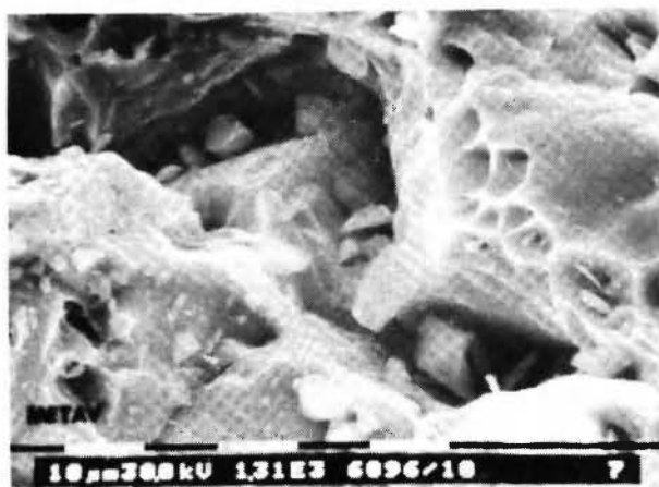
Fig. 7: Propagation of crack along the reinforcements distributed as bands in the over-aged composite.
