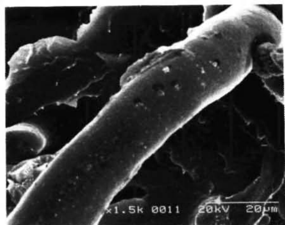
Fig. 7: Fracture surface of PET fiber-filled composites based on LDPE/PP blend matrix (50/50 ratio).
