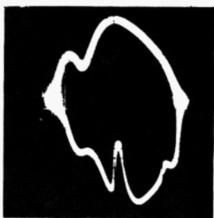
Fig. \partial \frac{dE}{dt} = f(E) curve of Congo Red indicator at the end point of the titration of \text{NH}_3 with \text{HAc} (a) just before and (b) at the end-point.
