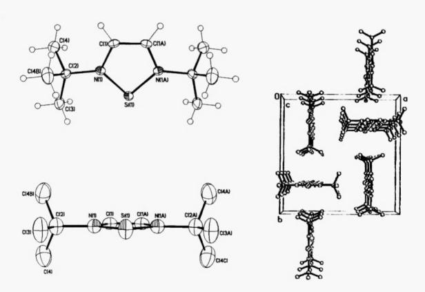
**Figure 1**. Molecular Structure of  $C_{10}H_{20}N_2Si$  (shown in two views). Displacement ellipsoids are plotted at the 50% probability level. Selected bond distances and angles: Si-N(1) 1.747(4), N(1)-C(1) 1.388(5), N(1)-C(2) 1.459(3), C(1)-C(1A), 1.320(8) Å; N(1)-Si-N(1A) 88.1(2), C(1)-N(1)-Si 112.4(3), C(1A)-C(1)-N(1) 113.6(2)°.
