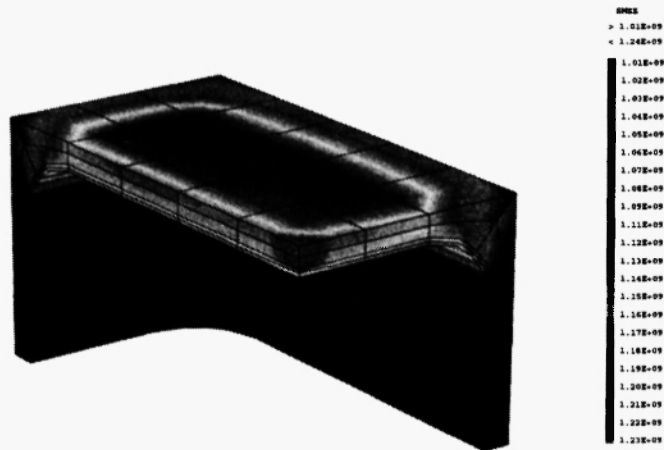
Fig. 16: \sigma_{33} stresses after traction to 2 % for raft microstructure of type N of AMI at 950°C ( \sigma_{33} in Pa).
