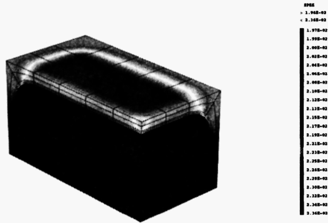
Fig. 13: \epsilon_{33}^P strains for rafts of type N of AM1 at 950°C.
