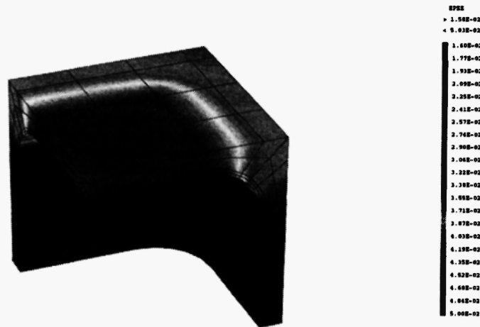
Fig. 5: Hydrostatic pressure distribution (in Pa), in the matrix, \gamma and \gamma' being viscoplastic.
