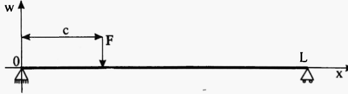
Fig. 2: Timoshenko's beam model
