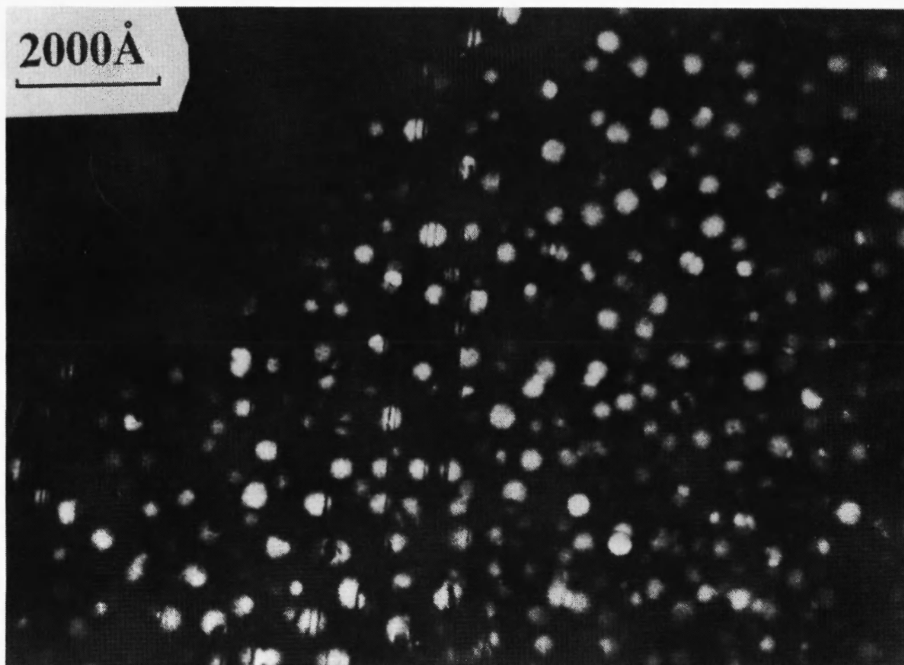
Fig. 7: Al 2.5 % Li alloys aged 45 hours at 195°C, fatigued in torsion ( \Delta\epsilon_t = 0.5\% ): sheared \delta' precipitates after fatigue, superlattice dark field [110], zone axis [110]
