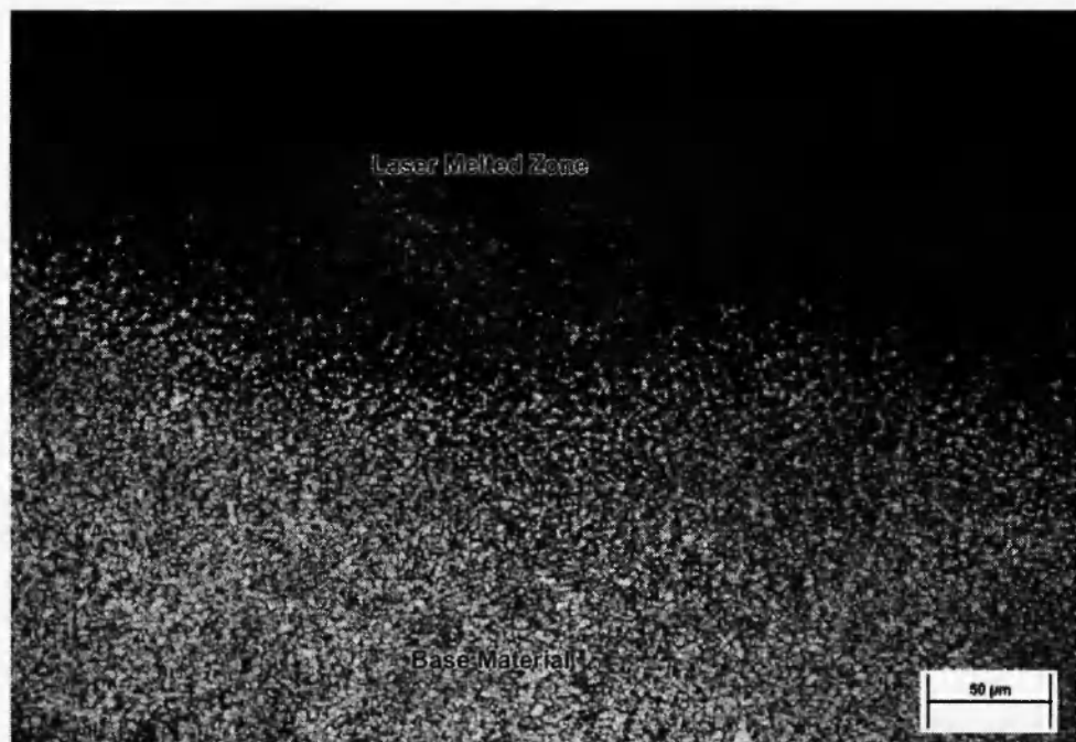
Fig. 5: Optical microstructure at energy density = 25 \times 10^6 \text{ J/m}^2
