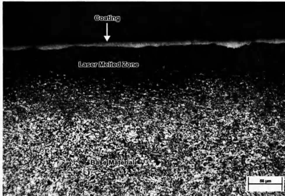
Fig. 4: Optical microstructure at energy density = 16 \times 10^6 \text{ J/m}^2
