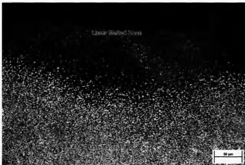
Fig. 6: Optical microstructure at energy density = 34 \times 10^6 \text{ J/m}^2
