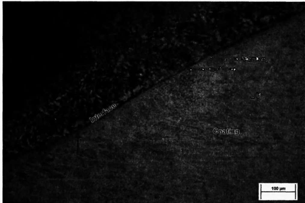
Fig. 8: Optical microstructure of coating interface at energy density = 47 \times 10^6 \text{ W/m}^2
