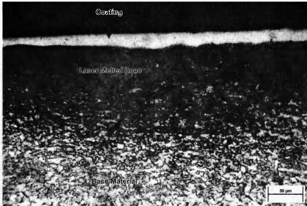
Fig. 3: Optical microstructure at energy density = 12 \times 10^6 \text{ J/m}^2
