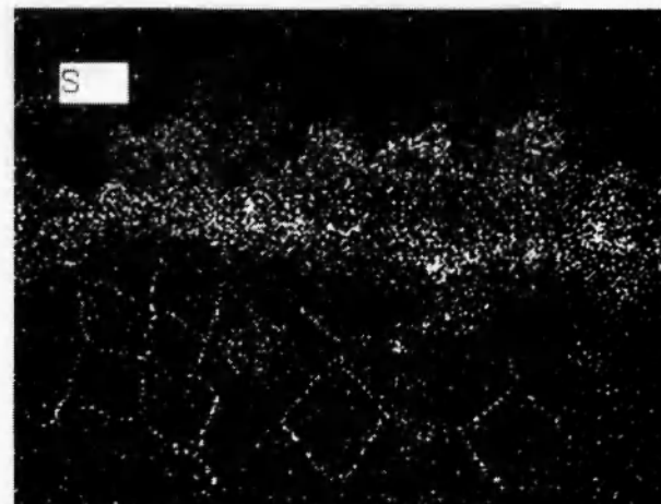
Fig. 9: Cross section of Fe-40Al-10Al 2 O 3 -0.2B corroded in Na 2 SO 4 at 1273 K. and X-ray mappings of Al, and S.
