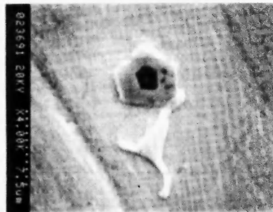
Fig. 7: Primary carbide particle nucleated on a TiN particle.
