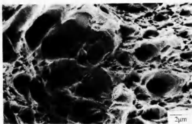
Fig. 5: Ductile dimple character of the fracture at 293 K
