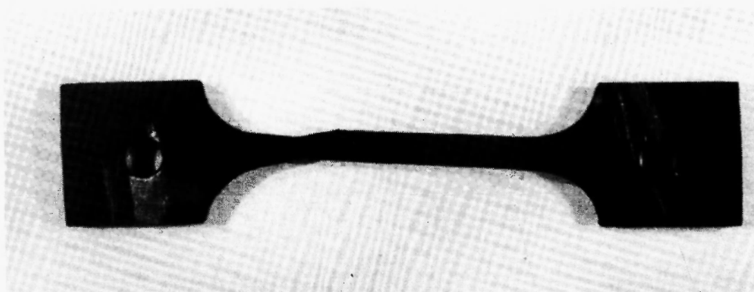
Fig. 9: Macro-photograph of an accelerated creep ruptured sample, tested at 112 MPa /923 K.
