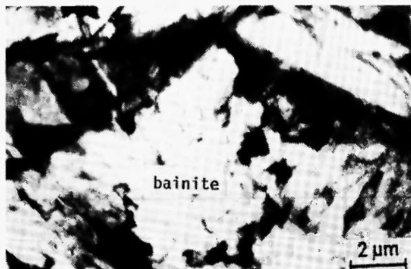
Fig. 2(a): Transmission electron micrograph of the initial microstructure of steel A showing laths of bainite.
