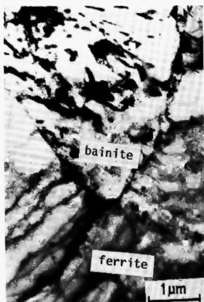
Fig. 2(b): Transmission electron micrograph of the initial microstructure of steel B showing granular bainite along with proeutectoid ferrite
