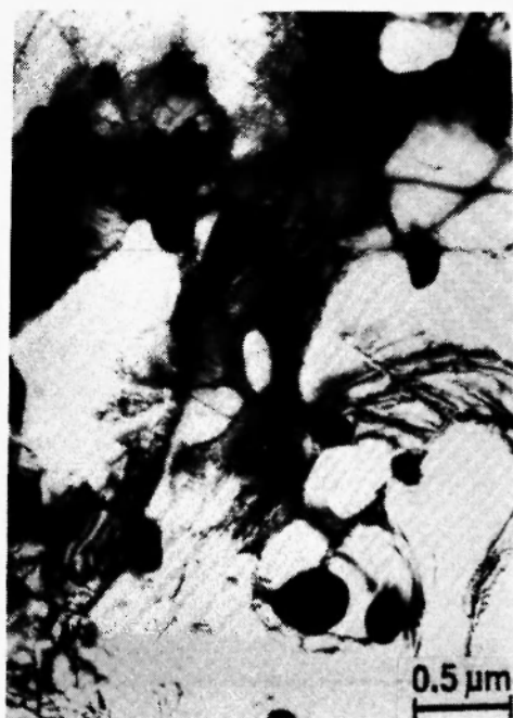
Fig. 5(a): Transmission Electron Micrograph depicting the globularisation of carbides and substructure formation in steel A when tempered at 1023K for 50h.
