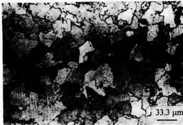
Fig. 2: A typical optical micrograph of service exposed main steam pipe of boilers at X 300, revealing ferrite grains dispersed with carbides. There is no evidence of graphitization and creep damage in the form of cavities and decarburization. This photomicrograph is for boiler D.
