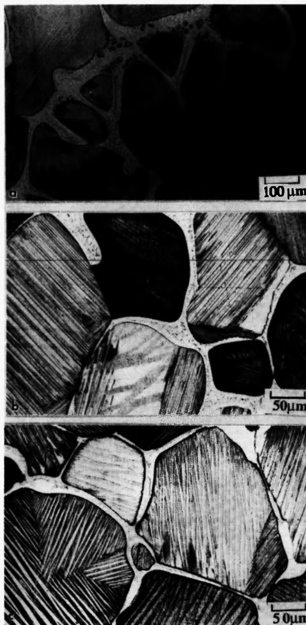
Fig. 1: Transverse microstructures (a) at quenched solid/liquid interface in the interdendritic region, (b) at the 5 mm below position of (a), and (c) at the 15 mm / below position of (a)
