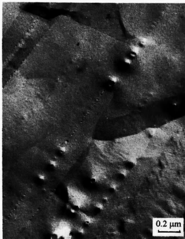
Fig. 11: Replication TEM micrograph showing long "secondary" bubble row formed by joining of the shorter "primary" ones. As a result of row-row collision and subsequent bubble coalescence, relatively large bubbles can form at the contact part of the original rows.
