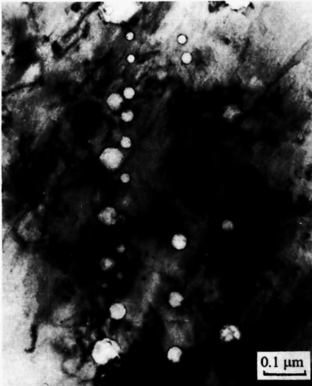
Fig. 5: TEM micrograph showing bubble rows situated close to each other.
