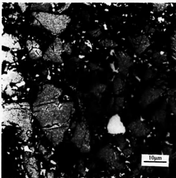
Fig. 5: The photomicrograph of the partially reduced \text{FeTiO}_3 sample ( X = 0.13 , 1085 K).
