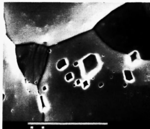
Fig. 3: Scanning electron micrograph showing grain boundary cavities growth from deformed-induced crack nuclei in undoped tungsten. The micron marker represents 10 \mu\text{m} .
