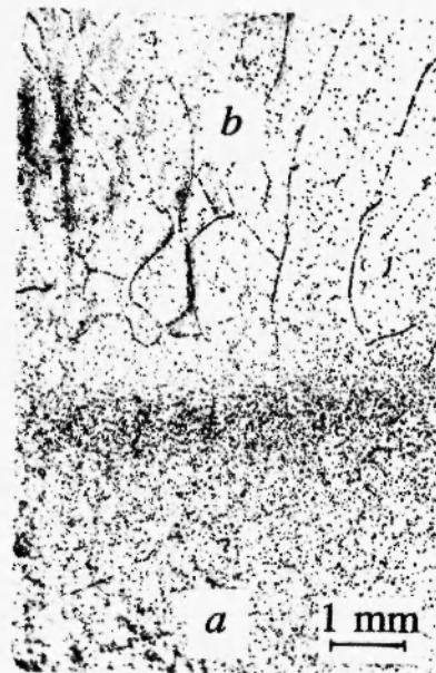
Fig. 8: Microstructure of W single crystal grown on the perfect monocrystalline seed. a - seed, b - grown single crystal.
