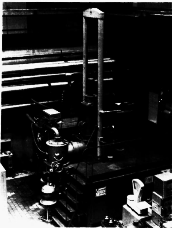
Fig. 1: Electron-beam floating zone melting furnace for purification refractory metals and for growing single crystals.
