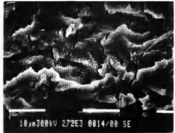
Fig. 11c: SEM fractograph of B3 specimens (base metal) in high \Delta K region.
