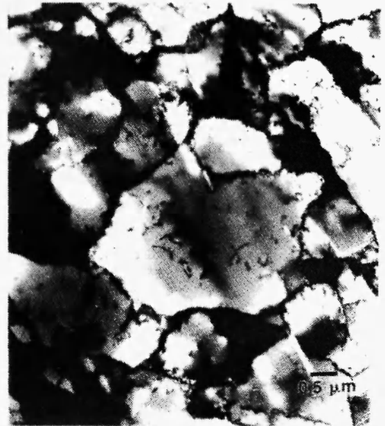
Figure 7b: TEM photomicrograph showing a longitudinal cross-section of the substructure of 2.67 mm diameter drawn wire which has been drawn at 1100 C. Subgrains are equiaxed, having an aspect ratio of 1.07. This indicates that polygonization did occur during drawing.
