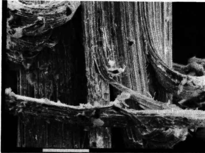
Fig.2. In the fracture zone the deep helical splits cause amazingly different deformation modes. (The mark denotes 100 \mu\text{m} .)
