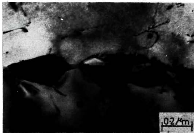
Fig. 3. Large M_{23}C_6 precipitates formed after final ageing at 973 K for 8 h.
