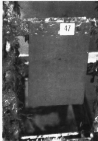
4.4. Disproportionated calcium resinate Dry film thickness required, minimum 200 \mu\text{m} Efficiency, 100 %
